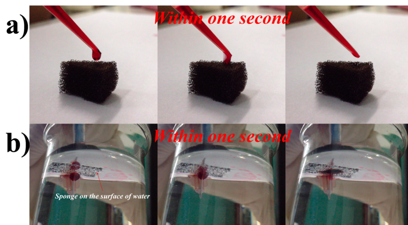
Figure 2. Contacting experiments of an oil droplet on the superhydrophobic sponge surface (a) in air and (b) under water.
